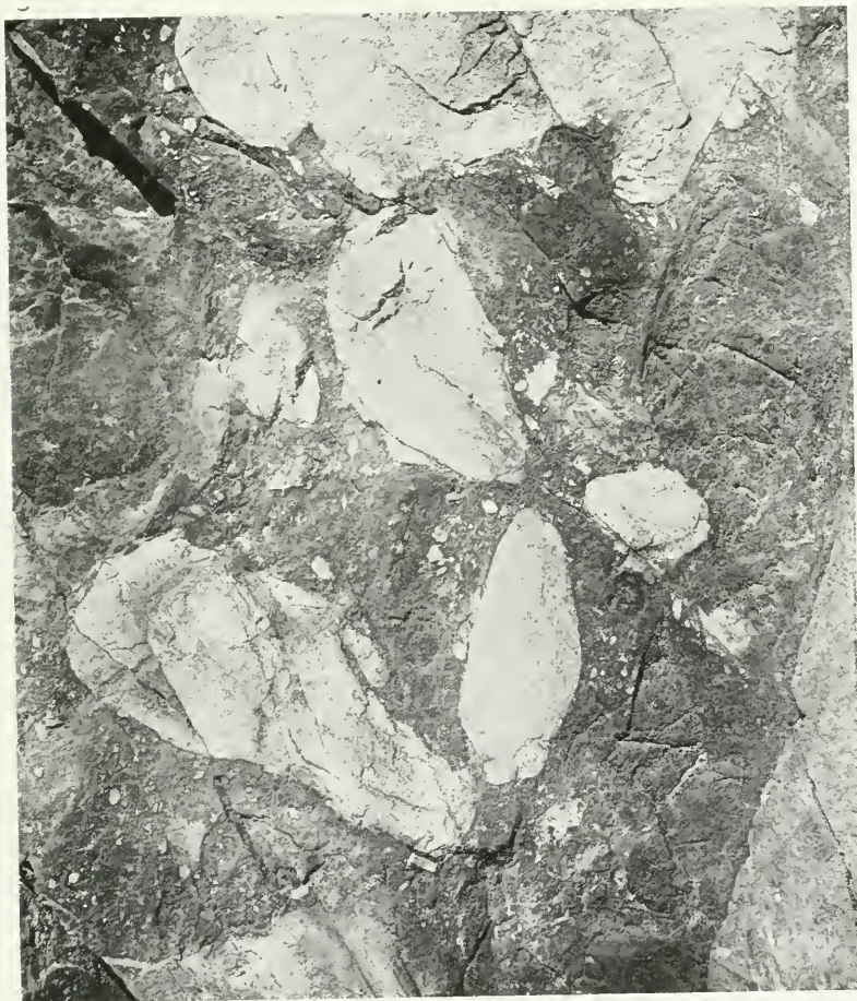
Fig. 4—Crush-conglomerate and crush-breccia, Copper Cliff, Sudbury area, Ontario. Width of face is 2 feet 6 inches. The rock has been formed by crushing and brecciation; the more finely crushed material constitutes the matrix for the larger fragments. The commercial ore bodies consist largely of these crushed rocks, but in the case of the ore bodies the matrix consists mainly of sulphides instead of the more finely crushed rock fragments, the more finely crushed rock having been partly or wholly replaced by ore.
